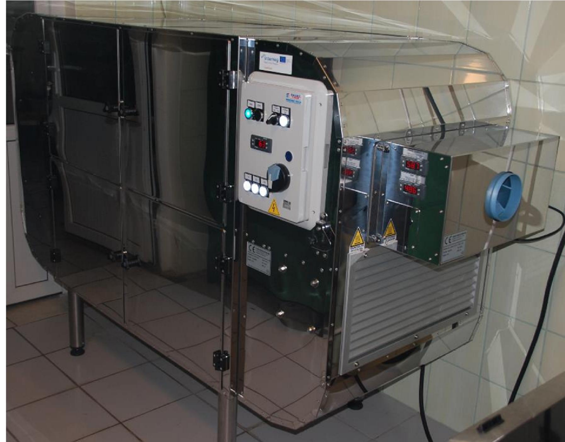
Equipment for drying of fruits, berries, vegetables and their processed products (incl. puree, pomace on silicone try).
