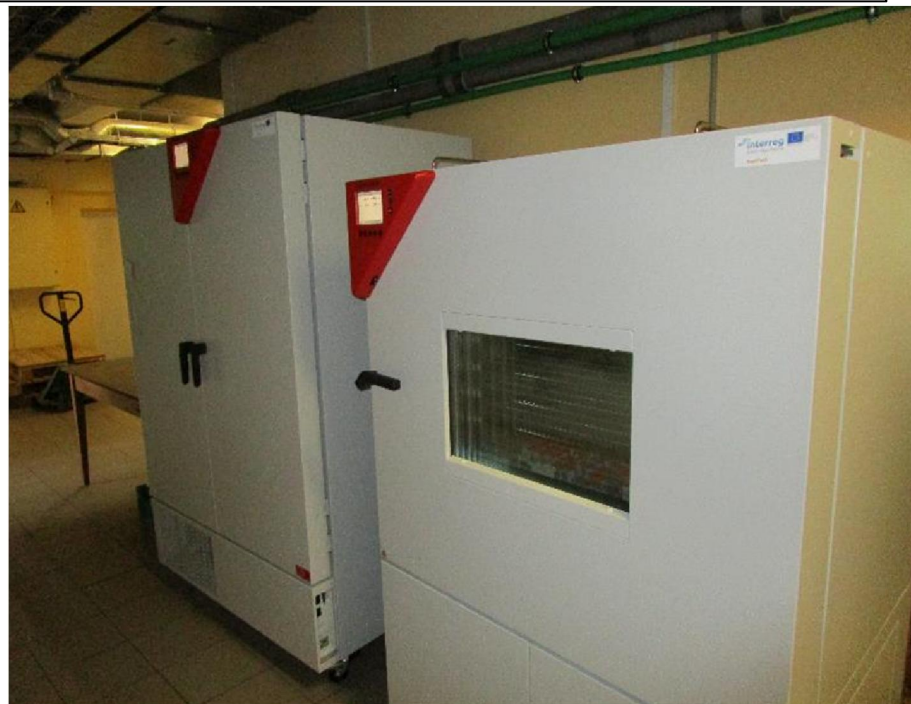
Climate and plant growing cameras for temperature stress examination
