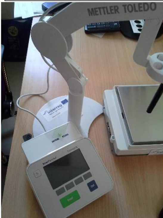
Conduktometer for relative elektrolyte leakage detecting
